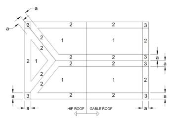
a: 10% OF LEAST HOIZONTAL DIMENSION OR 0.4h, WHICHEVER IS SMALLER, BUT NOT LESS THAN EITHER 4% OF LEAST HORIZONTAL DIMENSION OR 9FT (0.9M). OR AS DETERMINED BY DESIGN OR OTHER APPLICABLE CODE.
