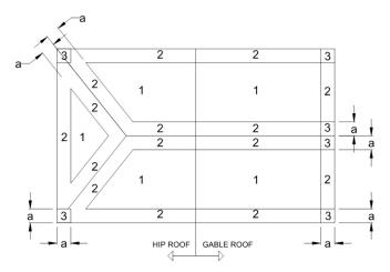
a: 10% OF LEAST HOIZONTAL DIMENSION OR 0.4h, WHICHEVER IS SMALLER, BUT NOT LESS THAN EITHER 4% OF LEAST HORIZONTAL DIMENSION NO 3 FT (0.9M). OR AS DETERMINED BY DESIGN OR OTHER APPLICABLE CODE.
