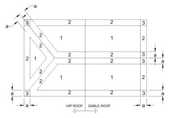
a: 10% OF LEAST HOIZONTAL DIMENSION OR 0.4h, WHICHEVER IS SMALLER, BUT NOT LESS THAN EITHER 4% OF LEAST HORIZONTAL DIMENSION OR 3FT (0.9M). OR AS DETERMINED BY DESIGN OR OTHER APPLICABLE CODE.
